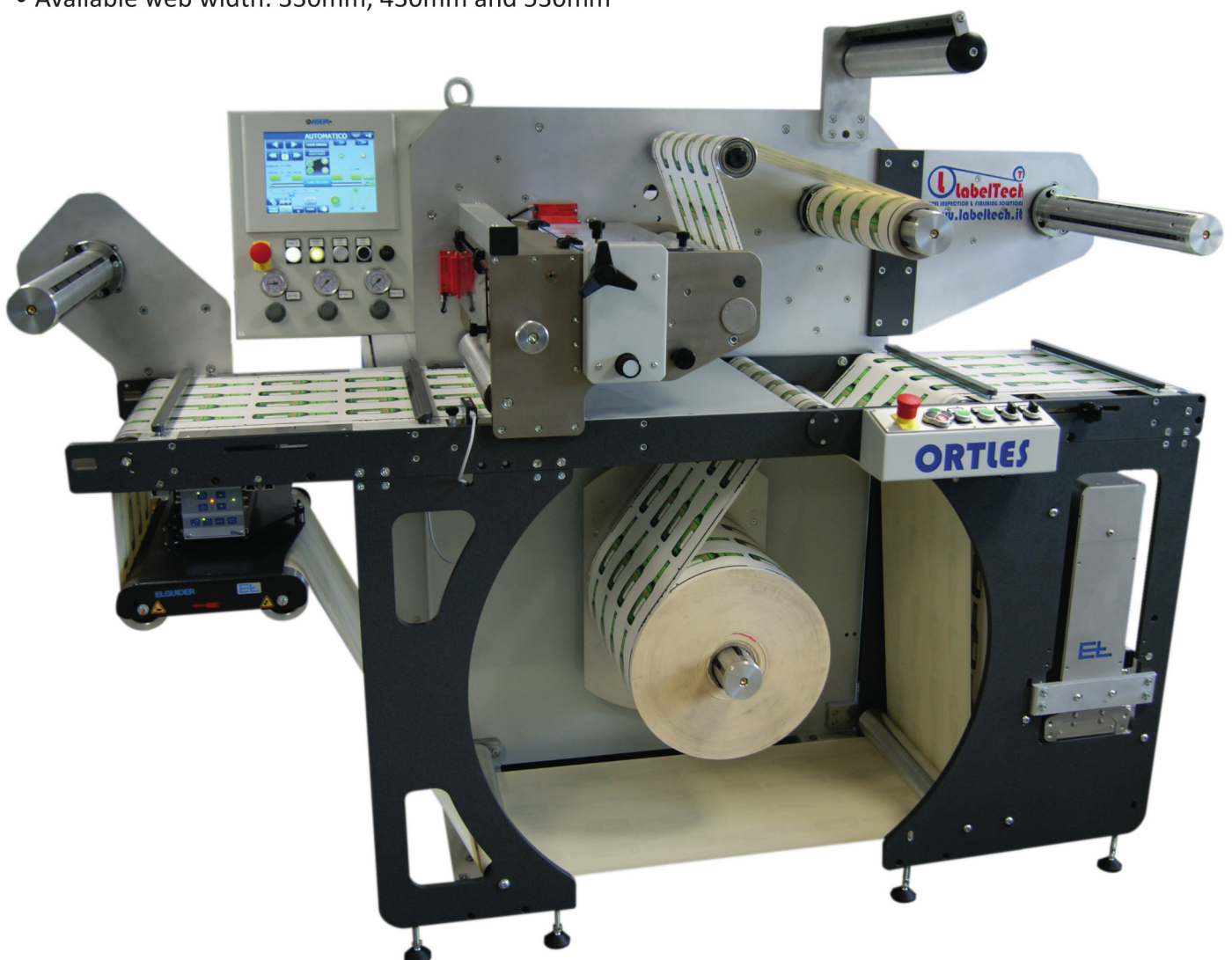
ORTLES 430 with dual rewriter, waste rewriter and quality inspection camera
