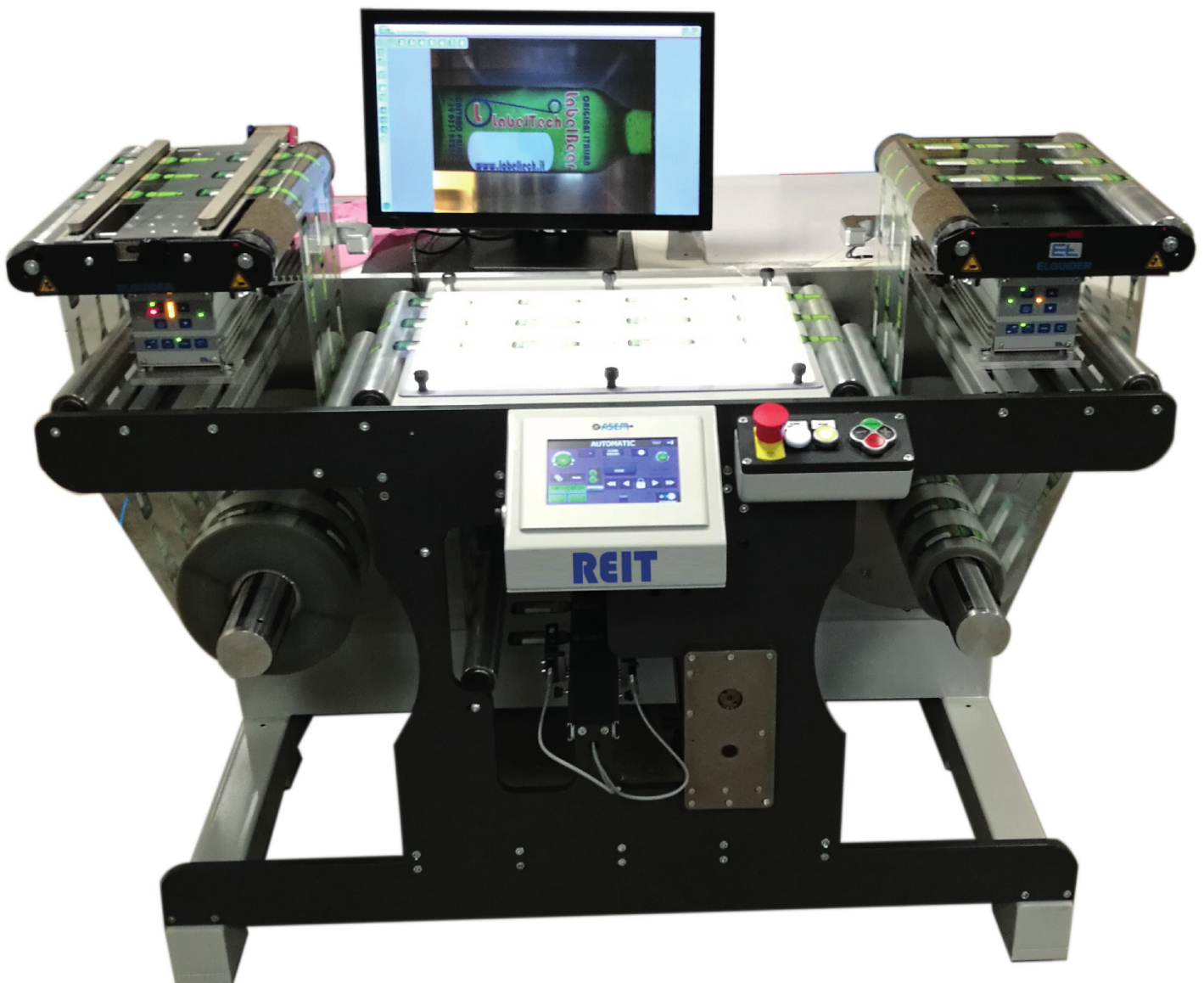
REIT doctoring rewinder with 2 web guides and inspection camera
